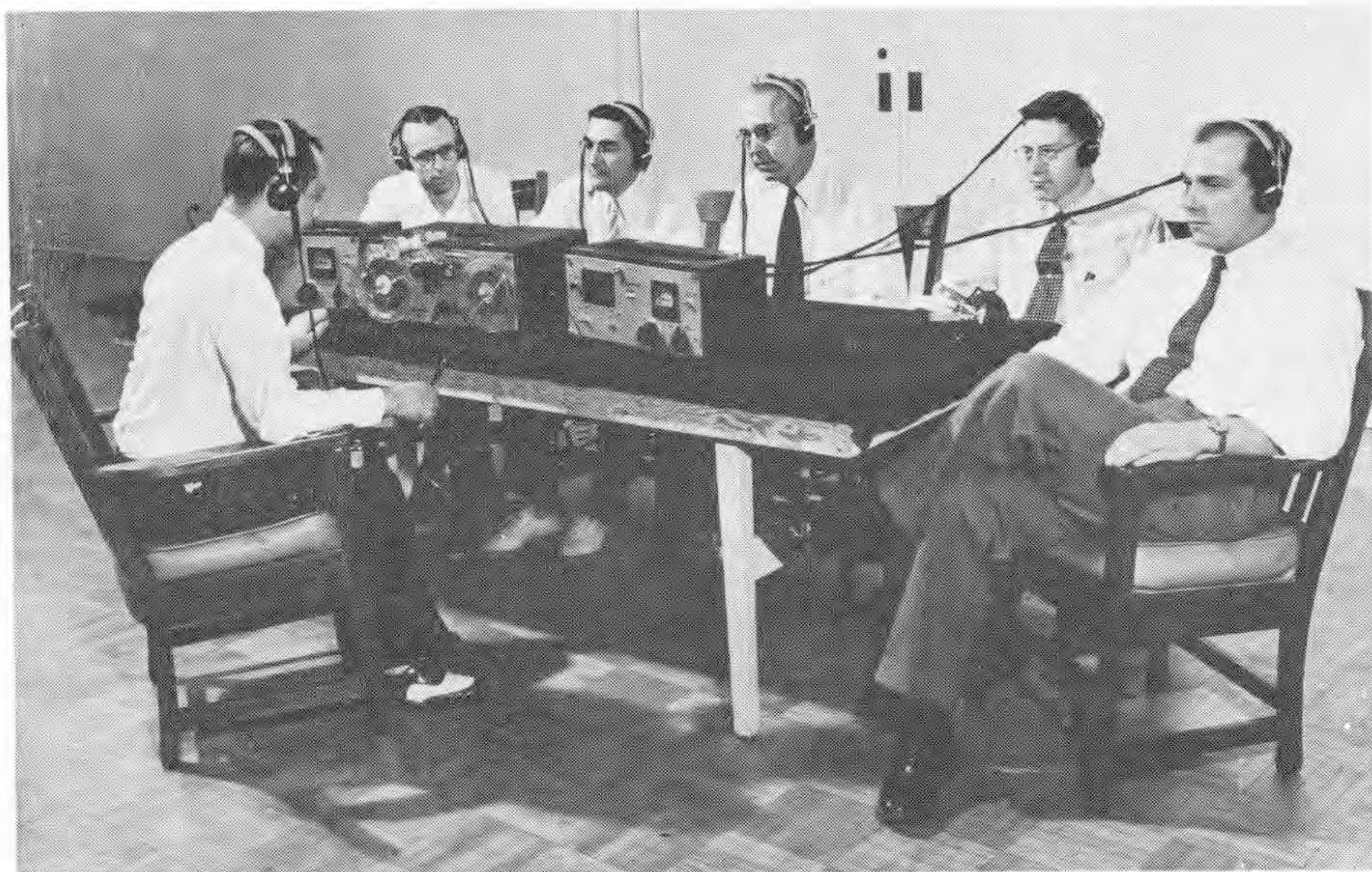
Norris Haight (left), head of the sound lab at the GM Proving Ground, plays a binaural magnecording of camshaft noises to a "jury" of five Oldsmobile engineers.
